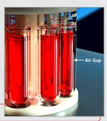
The patented SimAir® Test Cells, held in the (8) position SB+2 Carousel, utilize a unique air-gap between the test sample and the liquid bath medium to simulate the original air bath method.
