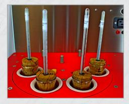
The SB+2 tests four (4) Cloud & Pour Point samples at a time. Accessories used with this Insert Module include Copper Sleeves, Glass Stators, Cork Rings & Discs, and Test Jar Stoppers.
