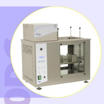
Stainless steel bath Calibration High precision ± 0.002°C Large windows 0.001°C readout **RS232** communication **Detachable front window**
